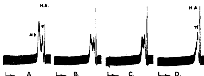
Fig. 2. The effect of varying the albumin content with a constant hyaluronic acid content on the Pi peak formation. A, 153 mg hyaluronic acid/100 ml + 480 mg bovine plasma albumin/100 ml \eta rel. 44 centipoises; B, 153 mg hyaluronic acid/100 ml + 360 mg bovine plasma albumin/100 ml \eta rel. 44 centipoises; C, 146 mg hyaluronic acid/100 ml + 280 mg bovine plasma albumin/100 ml \eta rel. 46 centipoises; D, 144 mg hyaluronic acid/100 ml + 250 mg bovine plasma albumin/100 ml \eta rel. 45 centipoises. Veronal buffer (pH 8.6) \mu = 0.1 . The intrinsic viscosity of the hyaluronic acid was 46 dl/g.
